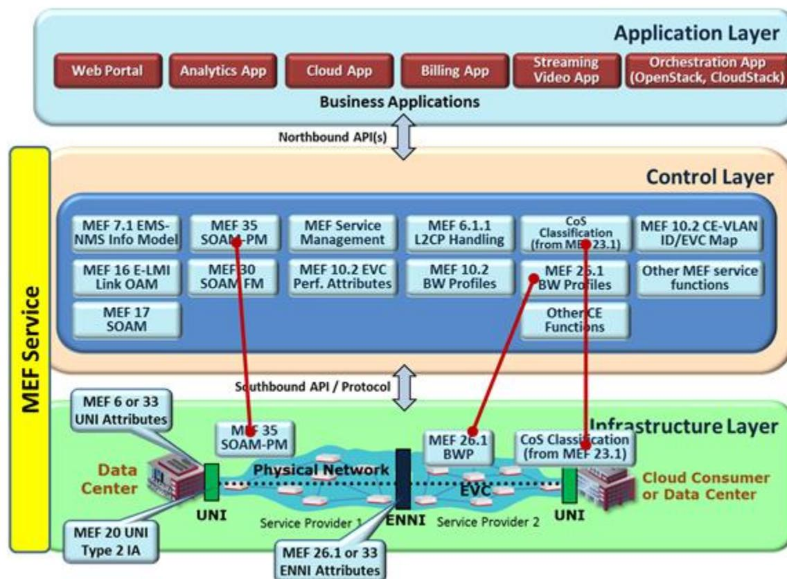
Figure 1: An example of mapping MEF specifications to Control and Infrastructure Layers
