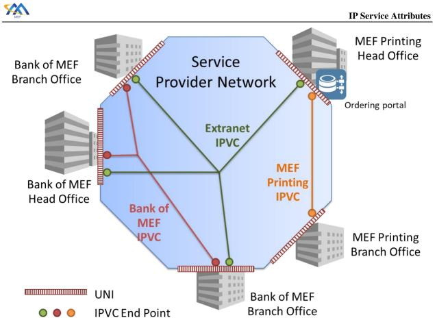
**Figure 10 – Extranet Example showing IPVCs**
