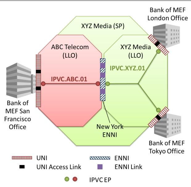
Figure 77 – Example Operator Services used for a Multipoint IP VPN
