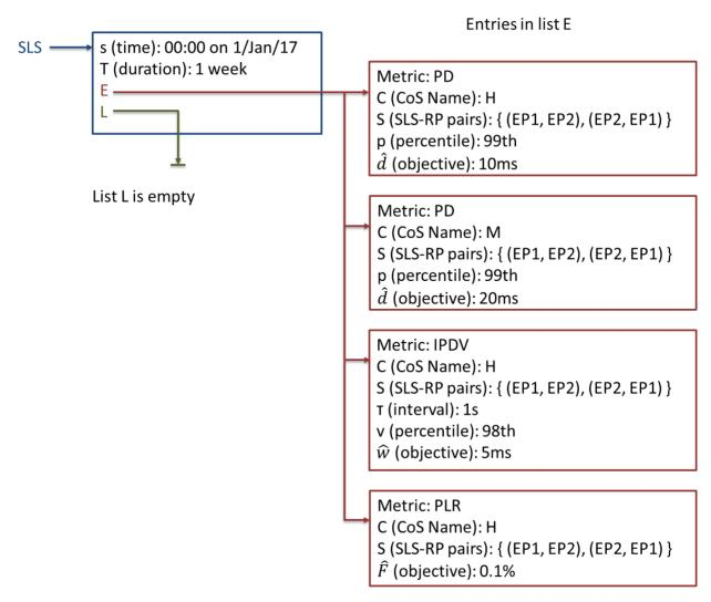
Figure 52 – Example SLS using IPVC EPs
