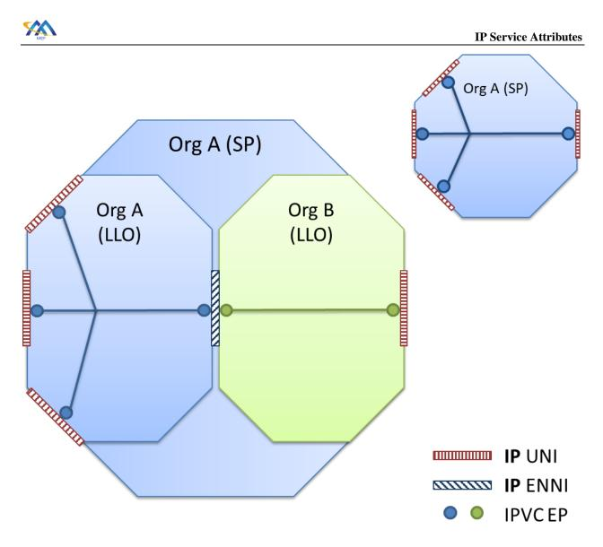
Figure 65 – Access to a Single Remote UNI
