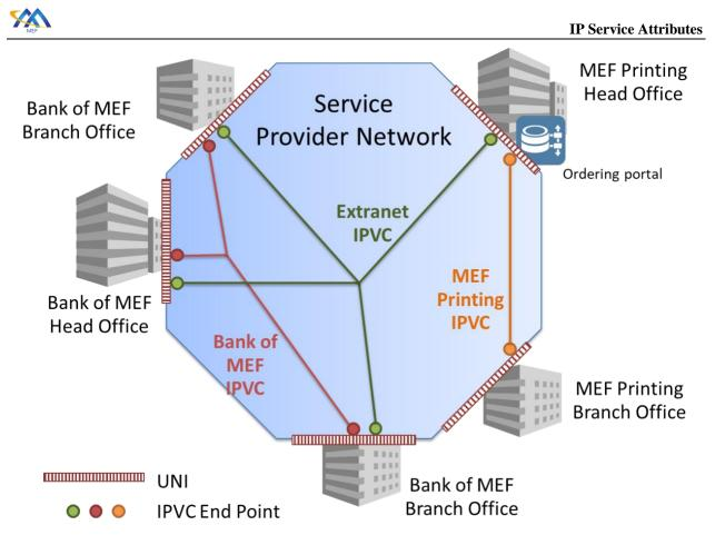
Figure 40 – Extranet Example showing IPVCs
