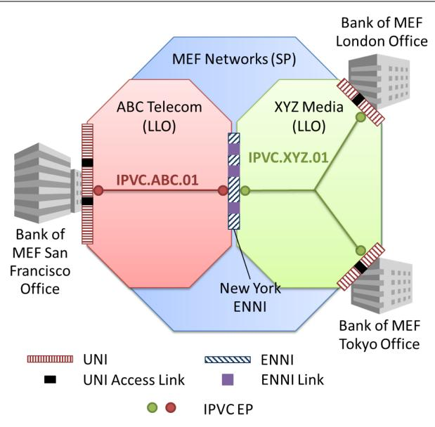
Figure 76 – Example Operator Services used for a Multipoint IP VPN
