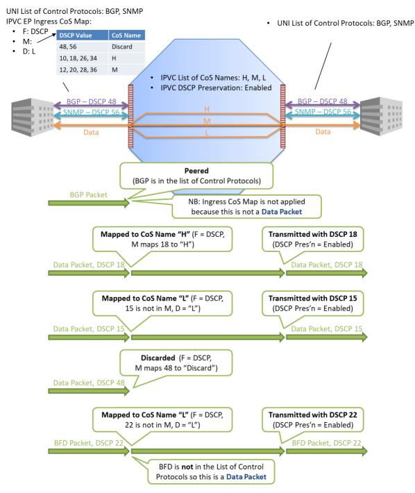
**Figure 48 – Example with DSCP Preservation showing packet handling**
