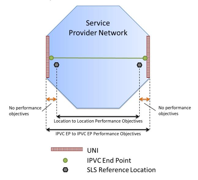
Figure 26 – Example of SLS specified using locations
