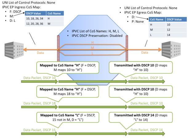
Figure 51 – Example of an Egress CoS Map showing packet handling
