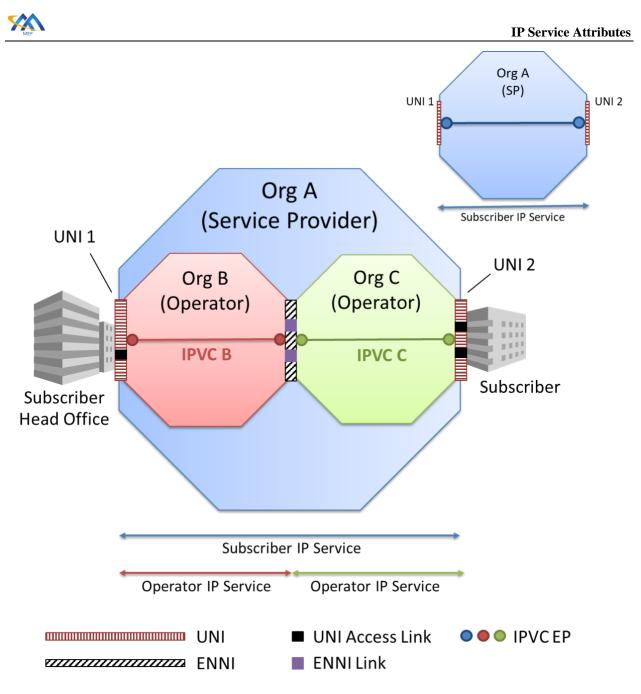
Figure 15 – Example showing Operator IPVCs
