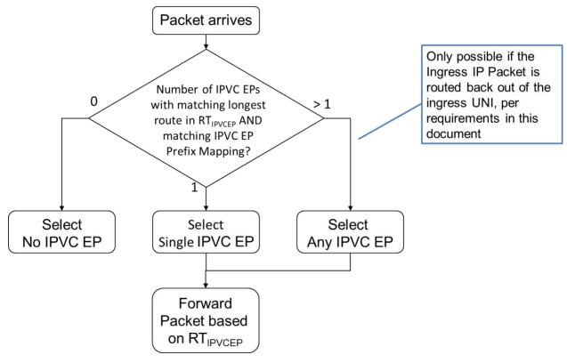
Figure 24 – Selecting an Ingress IPVC EP
