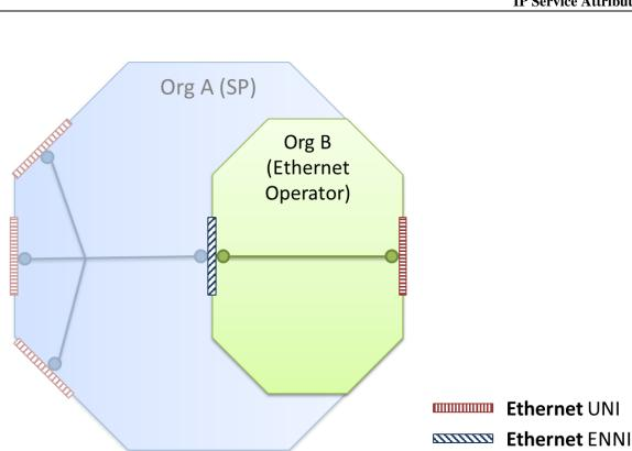
Figure 73 – Access E-Line connecting to an IP Service.
