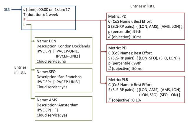
**Figure 53 – Example SLS using Locations**
