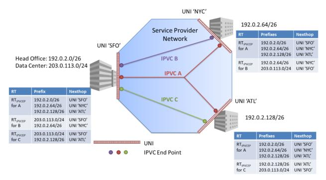
Figure 38 – Example IP Service – Per-IPVC EP Routing
