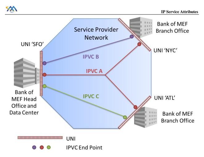
Figure 35 – Example IP Service Showing Three IPVCs
