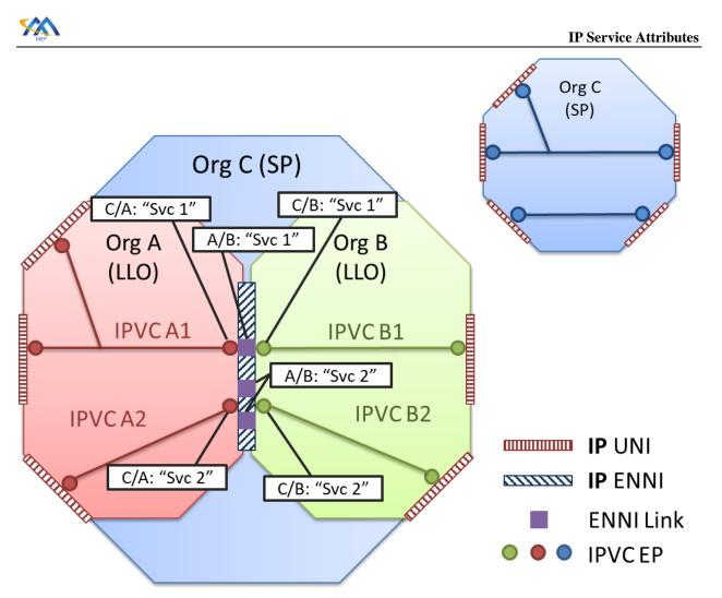
Figure 18 – Example of ENNI Service Mapping Identifiers for IP Services across an ENNI
