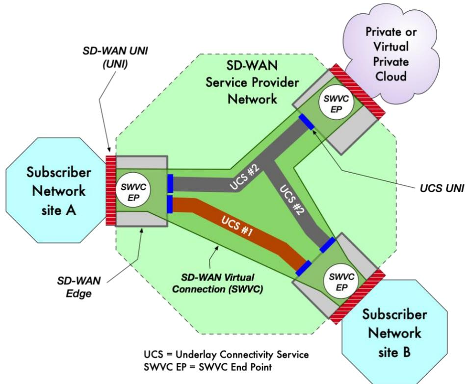
**Figure 1 – Components of an SD-WAN Service**
