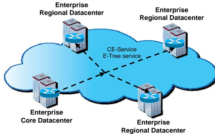
Figure 5 - Data Center Connectivity using an E-Tree CE service
