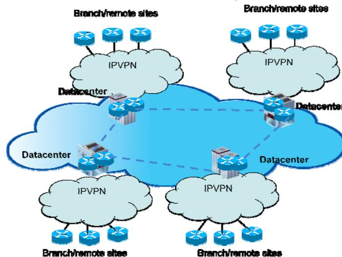
Figure 6: IP VPN for remote site to datacenter connection
