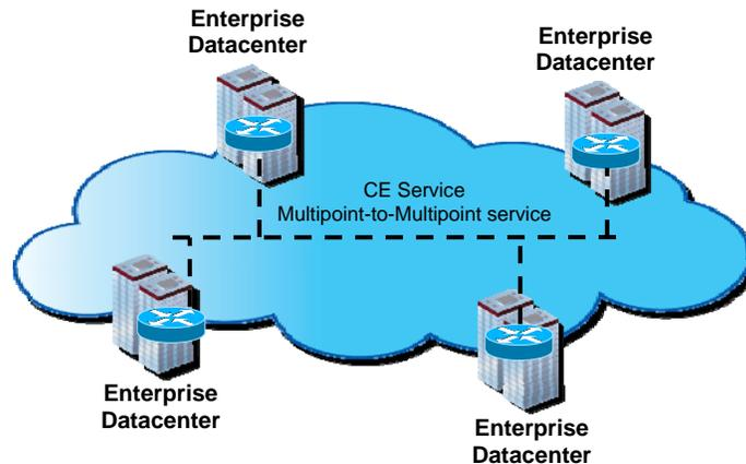
Figure 4 - Data Center Connectivity using an E-LAN CE service
