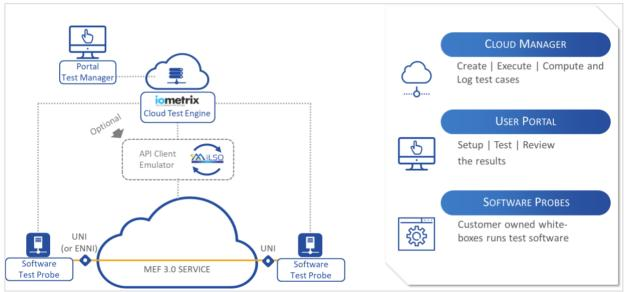
Figure 2 – MEF 3.0 CE Certification Test Environment
