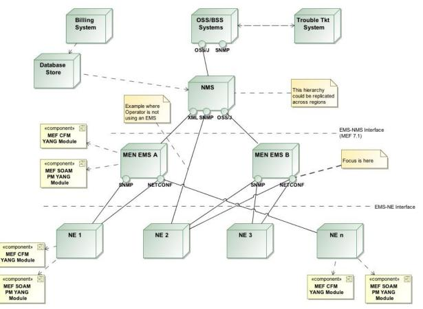
Figure 1 – Generalized OSS/BSS-NMS-EMS-NE Model
