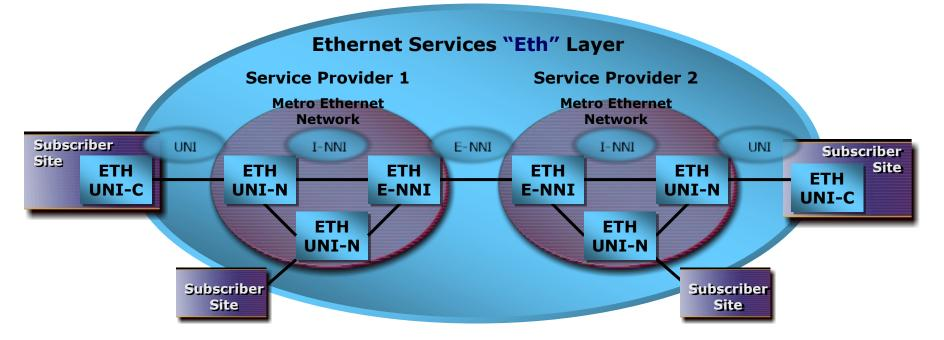
UNI: User Network Interface, UNI-C: UNI-customer side, UNI-N network side NNI: Network to Network Interface, E-NNI: External NNI: I-NNI Internal NNI
