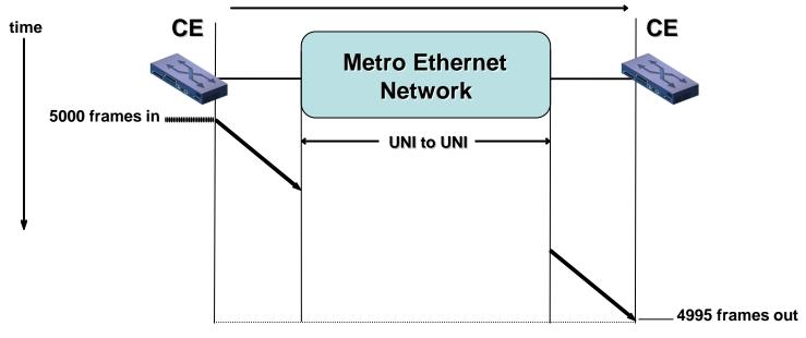
5 frames lost/or received as errored 0.1% Frame Loss Ratio (5/5000)
