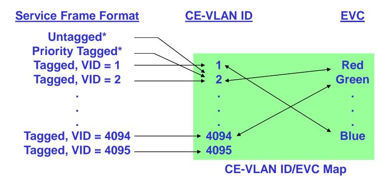
\*Untagged and Priority Tagged Service Frames can have the same CE-VLAN ID. (depends on use case) Configurable at each UNI. This is the behavior expected by an IEEE 802.1Q CE.
