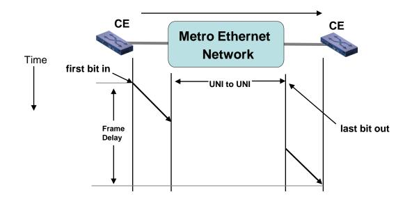
The One-way Frame Delay for an egress Service Frame at a given UNI in the EVC is defined as the time elapsed from the reception at the ingress UNI of the first bit of the corresponding ingress Service Frame until the Transmission of the last bit of the Service Frame at the given UNI. This delay definition is illustrated above
