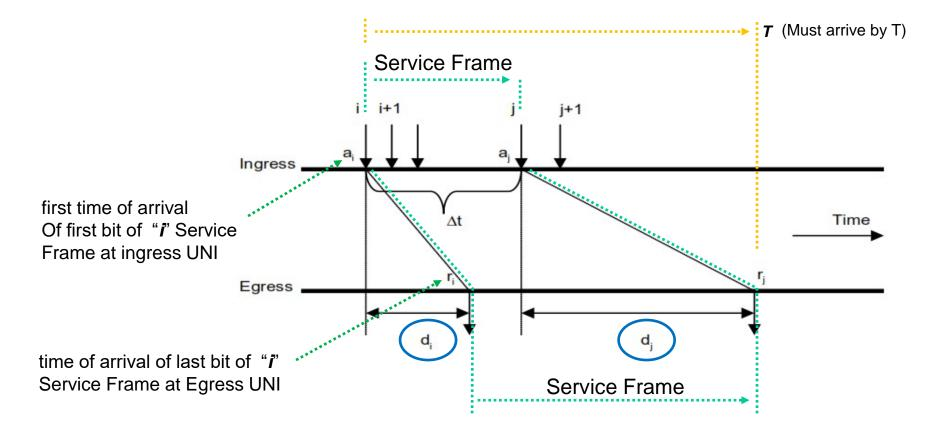
The difference in delays encountered by frame **i** and **j** is given by  $d_i - d_i$
