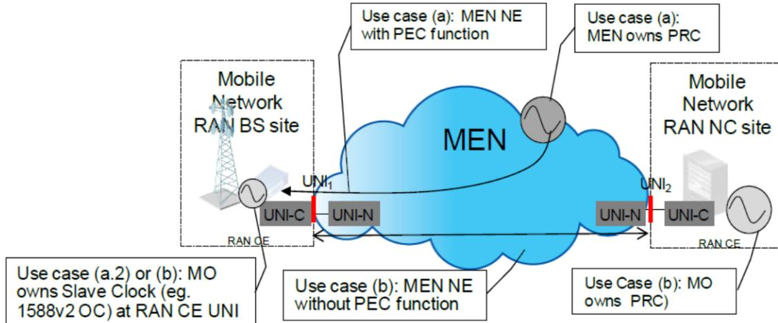
**Figure D – Packet Method to Distribute Reference Timing (Figure 21 of MEF 22.1[21])**
