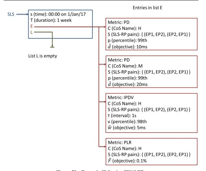
Figure 52 – Example SLS using IPVC EPs
