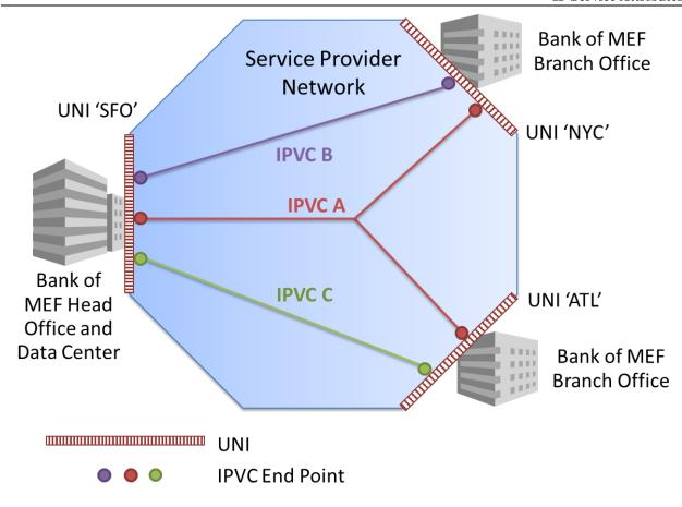
Figure 35 – Example IP Service Showing Three IPVCs
