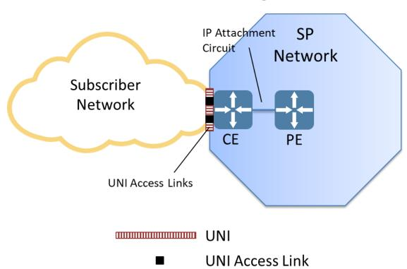
Figure 7 – Subscriber-managed and Provider-managed CEs
