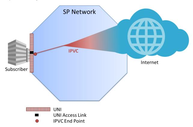
Figure 64 – Example Cloud Access IPVC for Internet Access
