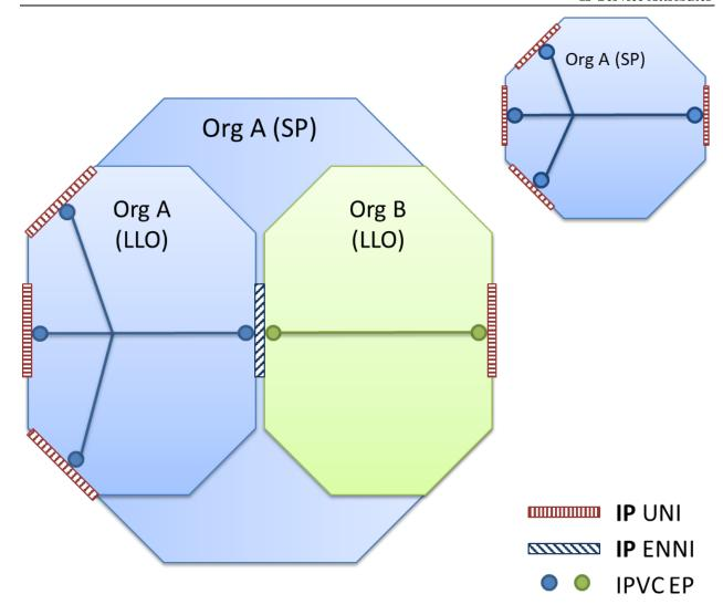
Figure 65 – Access to a Single Remote UNI
