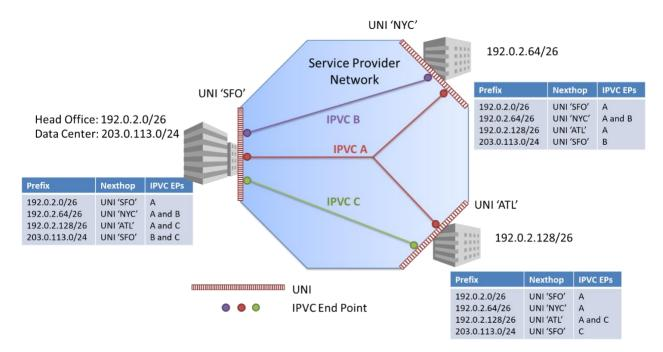
Figure 39 – Example IP Service – Combined Routing
