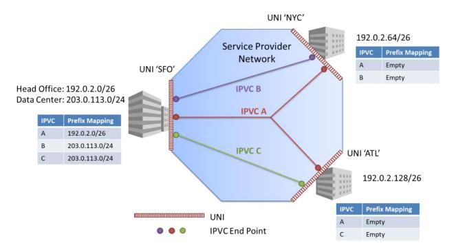
Figure 36 – Example IP Service – Subnets and Prefix Mapping
