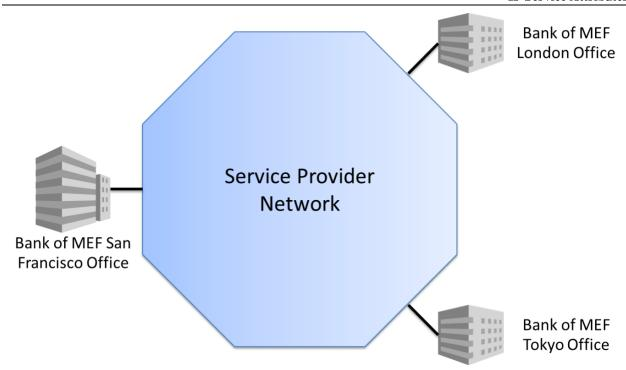
Figure 32 – Example of Multiple Subscriber Networks – Physical Topology
