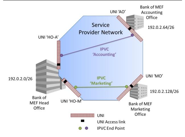
Figure 45 – Example IP Service showing IPVCs
