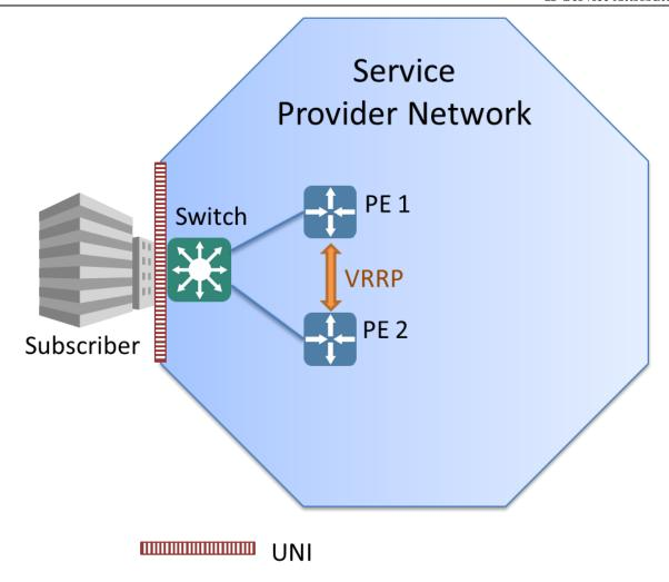
Figure 28 – UNI Access Link using VRRP
