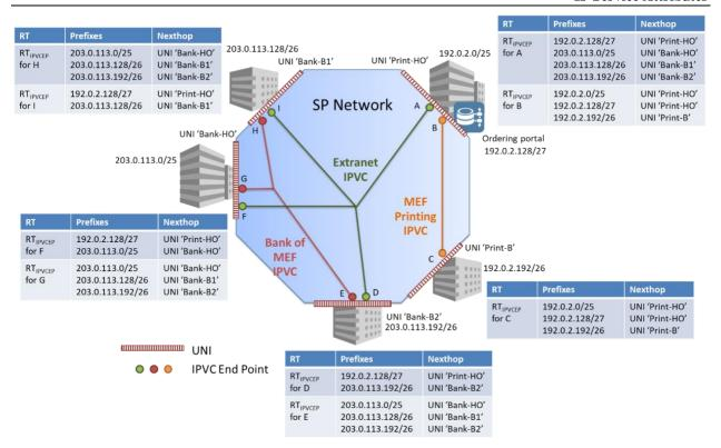
Figure 43 – Extranet Example showing Routing Tables
