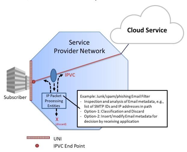
Figure 25 – Example of a Bump-in-the-Wire Service
