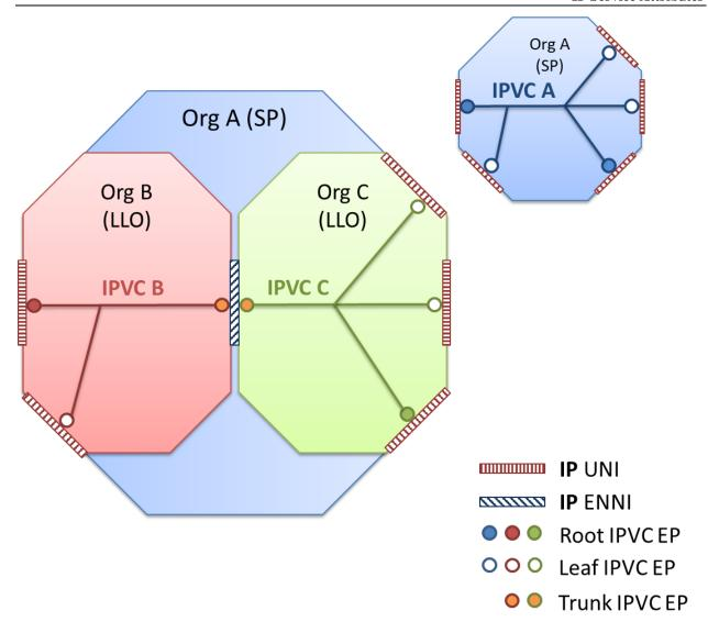
Figure 20 – Example of a Rooted Multipoint IPVC across an ENNI with Trunk IPVC EPs
