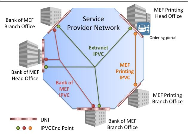
Figure 10 – Extranet Example showing IPVCs
