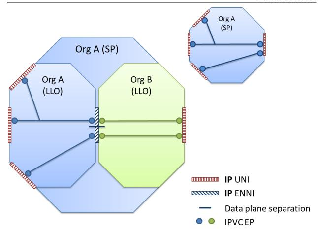
Figure 68 – Multiple Services at a Single Remote UNI
