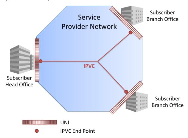
Figure 5 – Example of an IPVC and IPVC End Points
