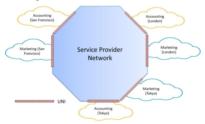
Figure 31 – Example of Multiple Subscriber Networks – Logical View
