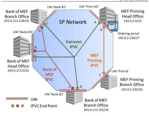
Figure 41 – Extranet Example showing IP Prefixes
