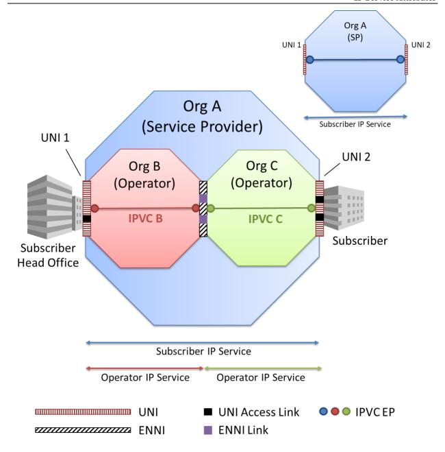
Figure 15 – Example showing Operator IPVCs
