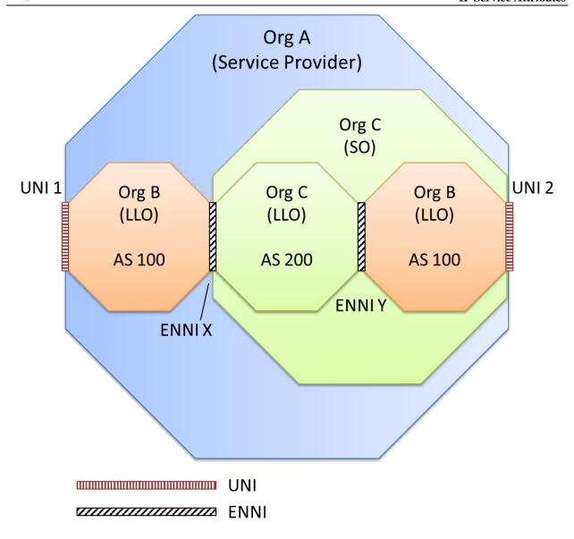
Figure 70 – Example of AS Override at an ENNI
