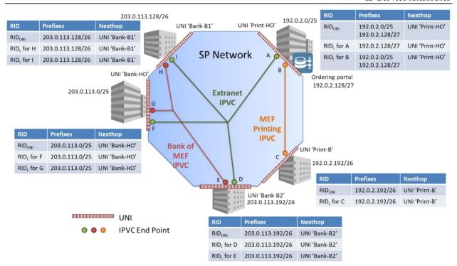
Figure 42 – Extranet Example showing Routing Information Databases
