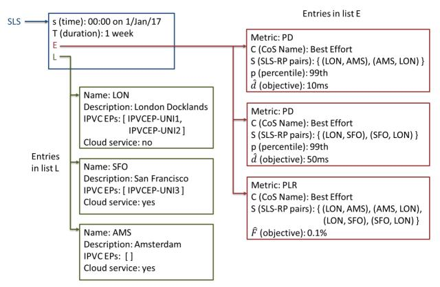
Figure 53 – Example SLS using Locations
