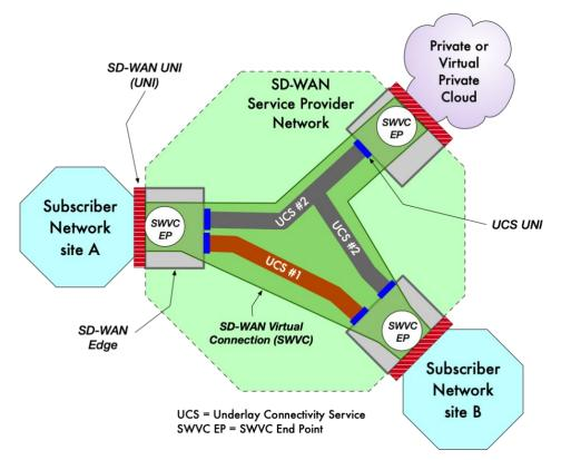
Figure 1 shows the SD-WAN Service components.
