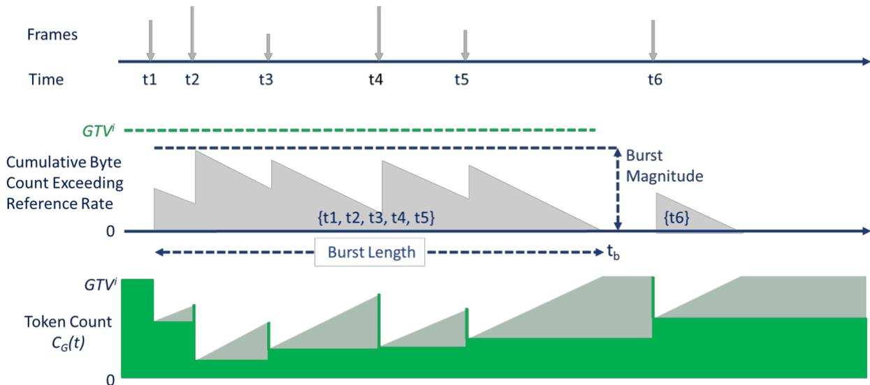
**Figure A1-2 – Token Request Sequence with a Burst Magnitude less than  $GTV_i$**
