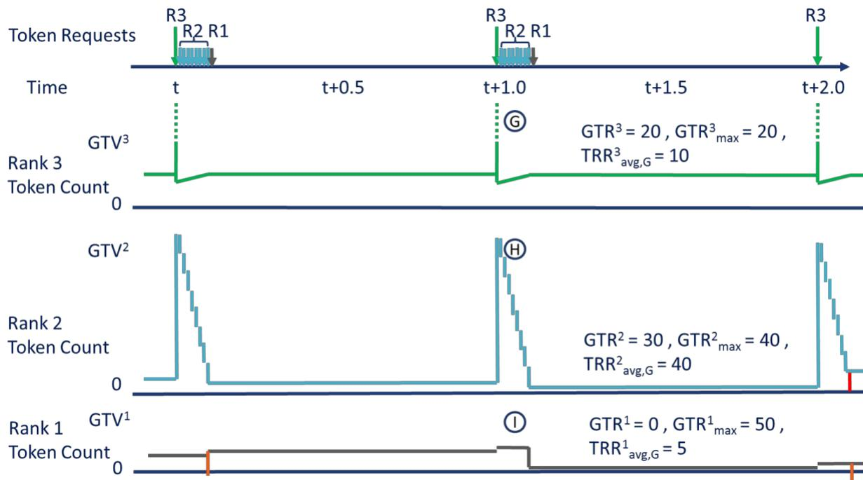
**Figure A1-6 – Transient Bypass Example Near Greatest Lower Bound**
