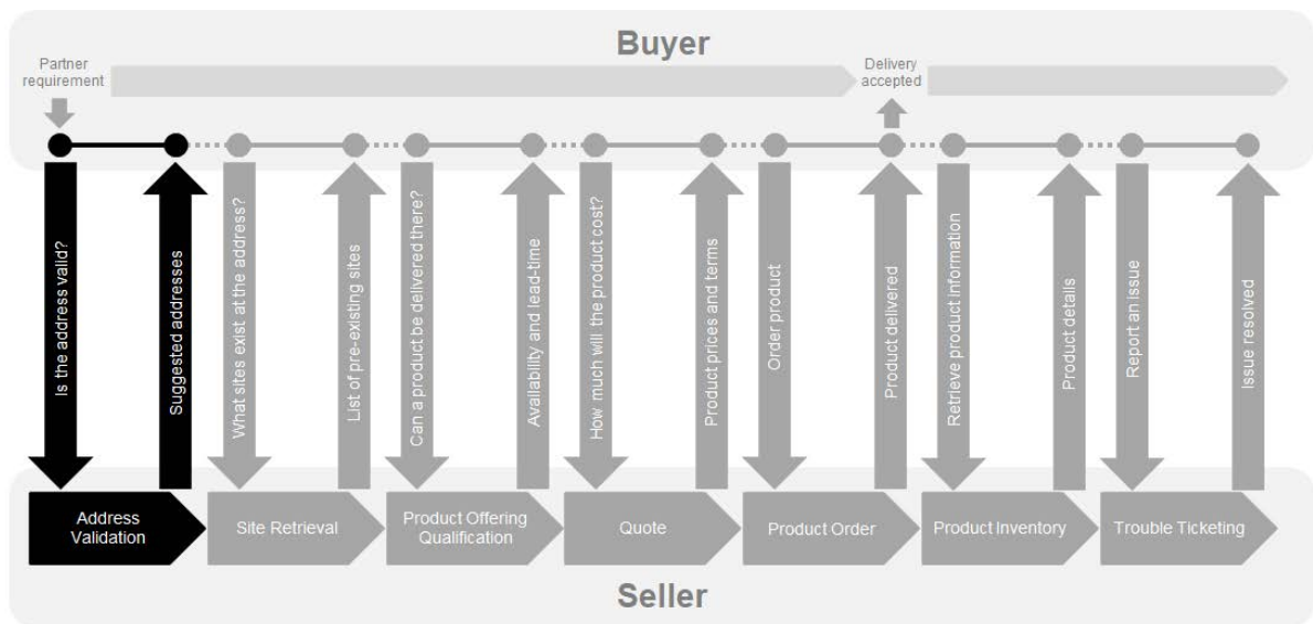
Figure 3. Cantata and Sonata End-to-End Function Flow
