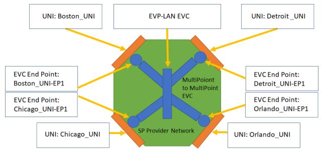
Figure A1-21 – UC2d: EVP-LAN Topology Diagram
