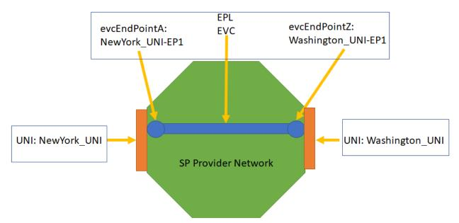
Figure A1-5 – UC2a: EPL Setup Diagram
