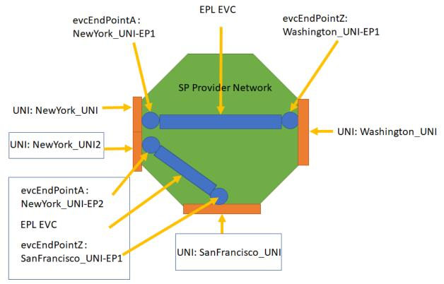
The topology of the Use Case 3a is presented in Figure A1-27. Newly added products are highlighted with a frame.
