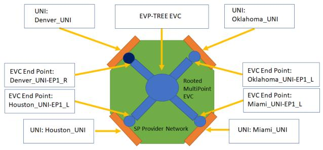
Figure A1-26 – UC2f: EVP-TREE Topology Diagram
