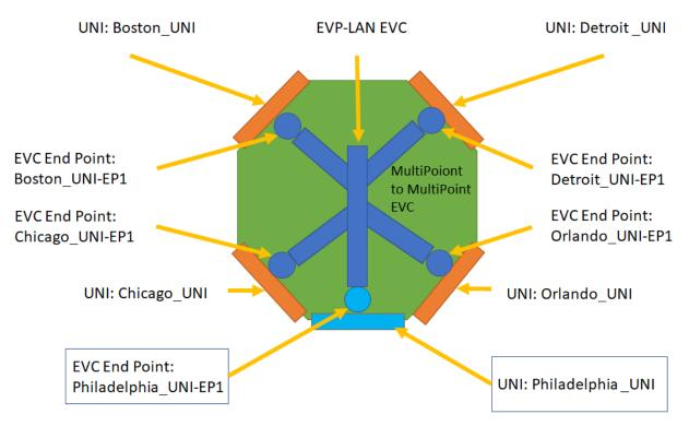
Figure A1-35 – UC7: EVP-LAN - add UNI and EVC End Point
