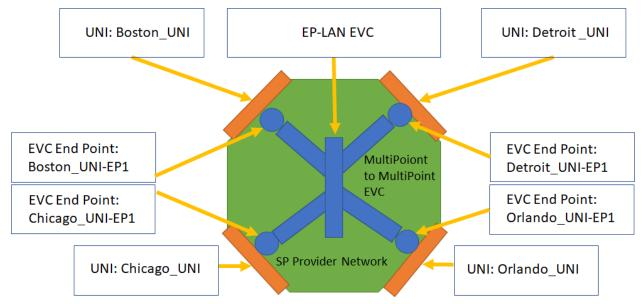
Figure A1-15 – UC2c: EP-LAN Setup Diagram
