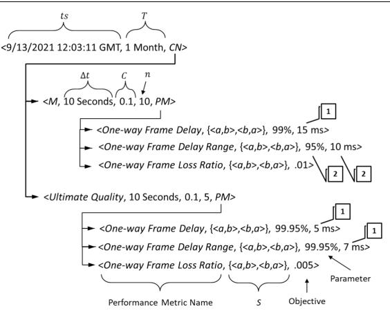
**Figure 6 – Value of the Service Level Specification for the EVC**
