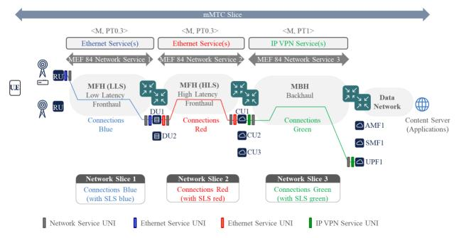
Figure 5 – Example Network with Network Services and Connectivity Services
