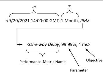
Figure 7 – Value of the Service Level Specification for the Subscriber L1VC
