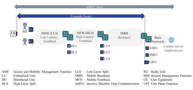
**Figure 4 – Example Network Prior to Network Services**
