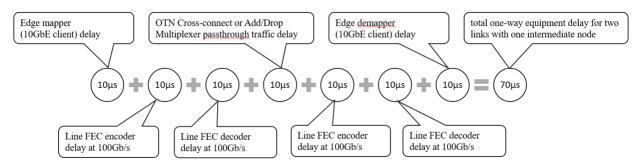
Figure 3 – Example Equipment Delays for Two Links with One Intermediate Node
