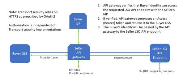
Figure 4 – Example Authorization Framework using Seller's IdP
