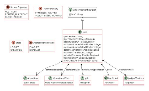
Figure 6. A simplified view on IPVC service specification data model
