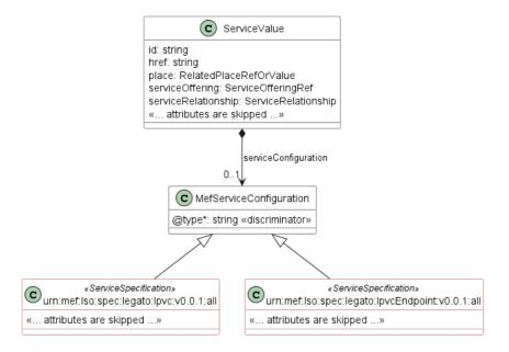
Figure 5. The Extension Pattern with Sample Service-Specific Extensions
